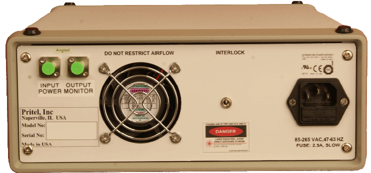
LNHP-PMFFA-xx model with Input/Output power monitor option
